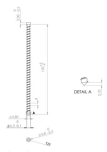
Figure 11. Concrete screw 6.5 x 150
