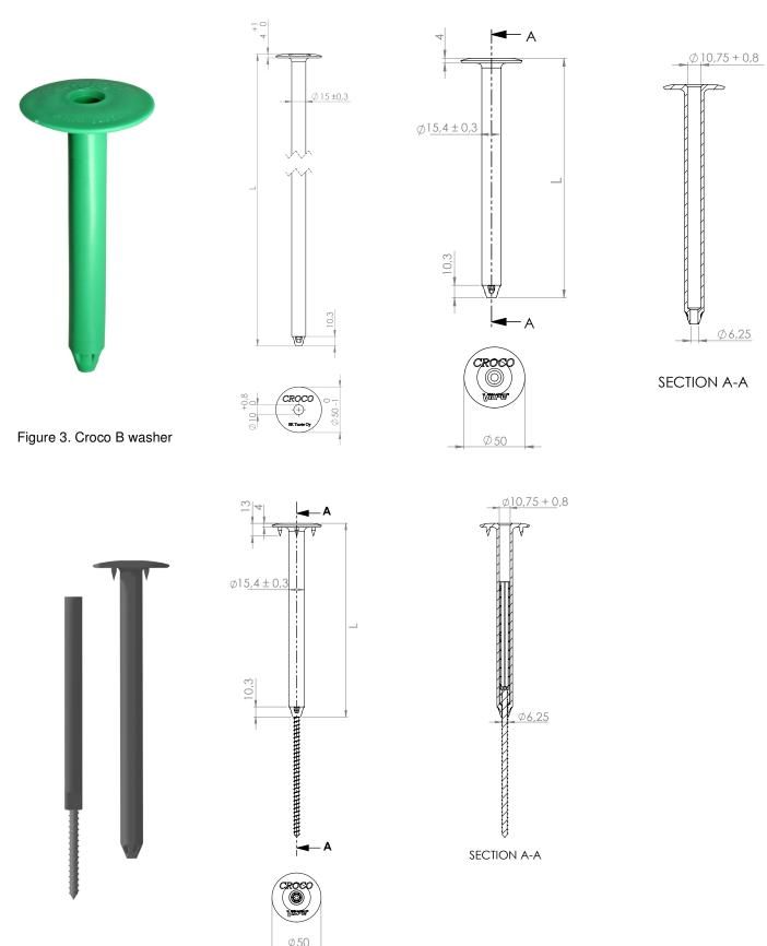
Figure 4. Croco A Adjustable Fastener
