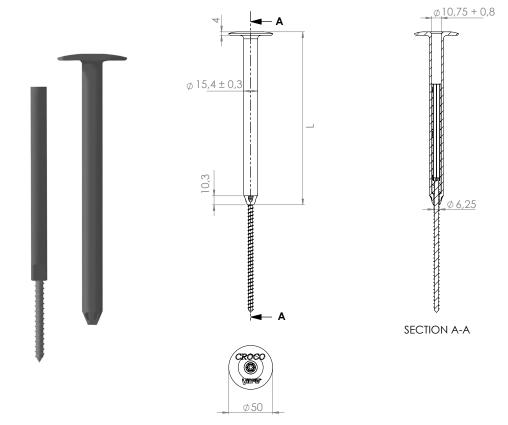
Figure 5. Croco B Adjustable Fastener
